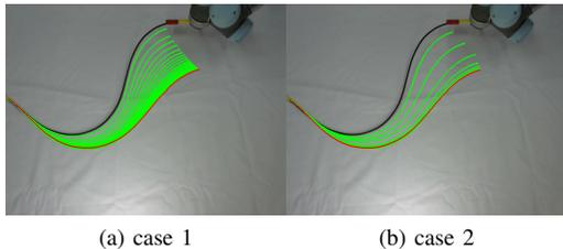
Fig. 21. Initial (black solid line), transition (green solid line) and target (red solid line) configurations between two conditions (case 1:  $\omega_1 = 0.01, \omega_2 = 0.99$  and case 2:  $\omega_1 = 0.99, \omega_2 = 0.01$ ) of JEU (44) tested in the LKF.
