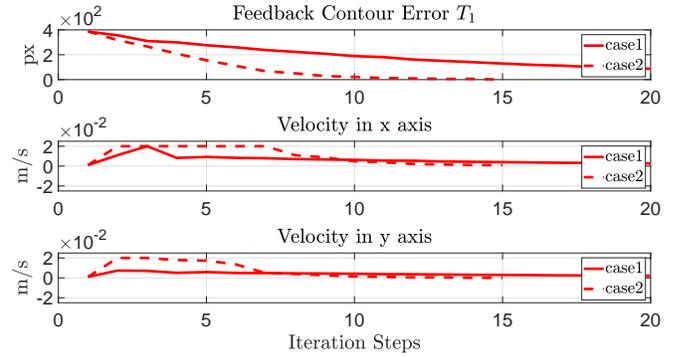
Fig. 22. Profiles of the cost function  $T_1$  and velocity command  $\Delta \mathbf{r}_k$  between two different weight values (case 1:  $\omega_1 = 0.01, \omega_2 = 0.99$  and case 2:  $\omega_1 = 0.99, \omega_2 = 0.01$ ) of JEU (44) tested in the LKF.
