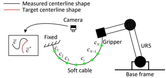
Fig. 1. Representation of the cable manipulation case of study, where a vision sensor continuously measures the feature vector  $\mathbf{s}$  of the cable, which should be accurately deformed into target feature  $\mathbf{s}^*$  within the controller.
