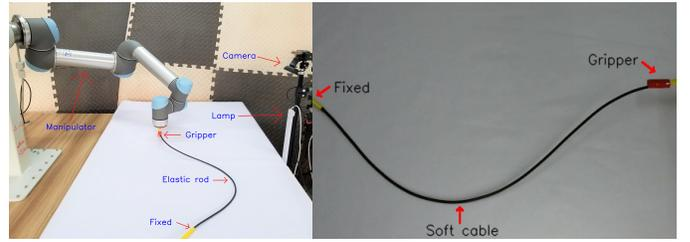
Fig. 11. Experimental setup.
